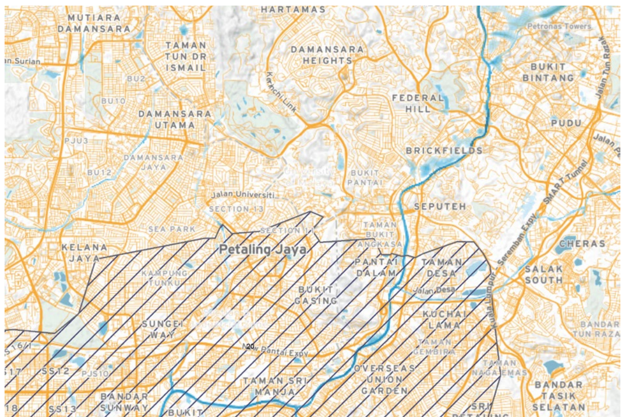
Figure 2 Example of defended river area data for Malaysia with a standard of protection of 20 years (hashed polygons) overlaid on top of the 20-year return period river flood map (blue). The overlap between both datasets indicates areas that benefit from existing flood defences during river flood events of return periods of up to 20 years.
