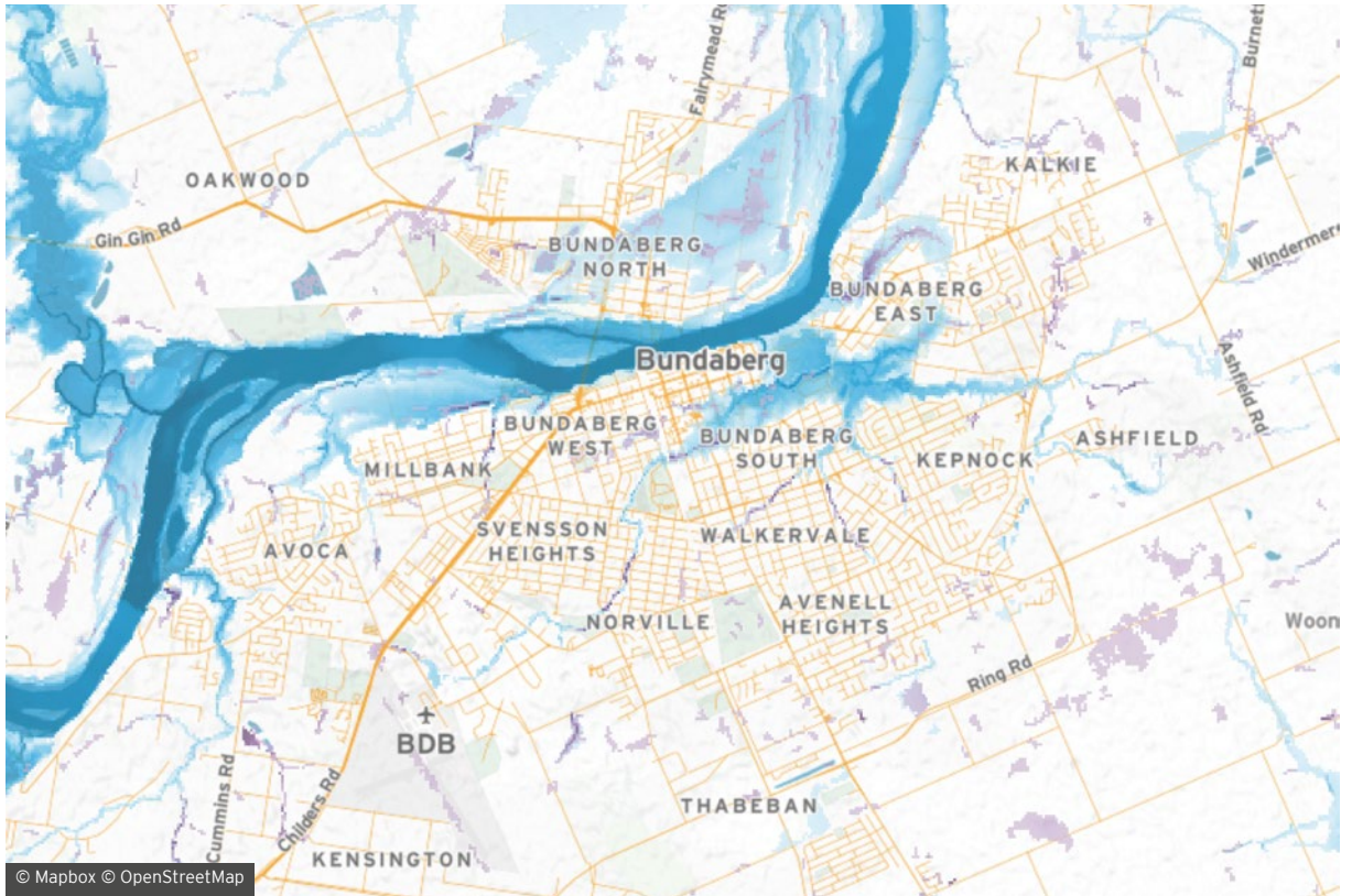
Figure 1 30m flood map extents for the 100-year return period, Bundaberg, Australia. River flood (blue) and surface water flood (purple).
